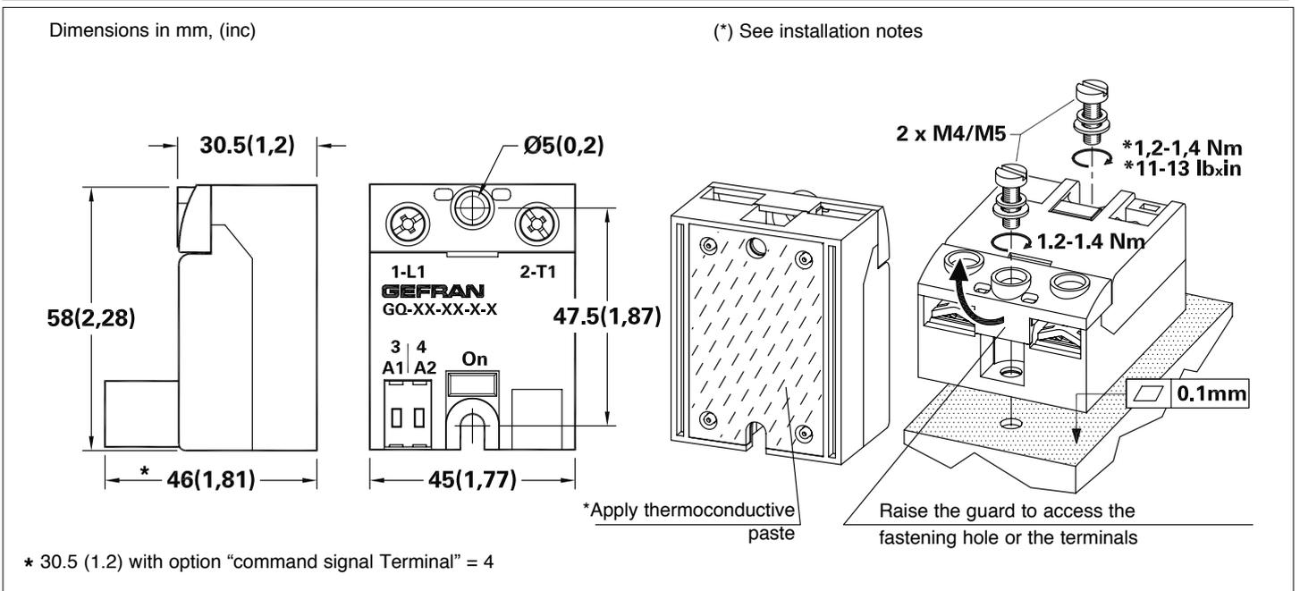
Alternately tighten the two fastening screws until reaching a torque of 0.4...0.6 Nm. Wait 5 minutes for any excess paste to run off.
