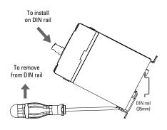
fig. 1 SSR mounted on DIN rail
