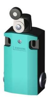
SIRIUS POSITION SWITCH 3SE5162, METAL ENCLOSURE XL,56MM WIDE WITH TWIST LEVER 27MM, FROM METAL AND PLASTIC ROLLER 19MM DEVICE CONNECTION 3X(M20X1.5), 2X (1NO/1NC ) SNAP-ACTION CONTACTS; IP66/ IP67
