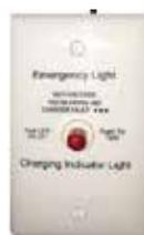
PLRTS is an optional test switch that includes a wall plate for a single gang J-box. Only one LBU7-M/M2 series emergency driver can be wired to each PLRTS switch at a time. Remote switch is intended to be used in place of the internal switch supplied with the driver. Use Class 2 wiring methods for installing switch and wiring. Switch wire length can be 50ft maximum from the emergency driver.
