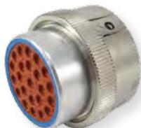
The HDB is designed to provide an emergency disconnect between farm tractors and implements that require power connections. The HDB breakaway plug is designed to break the connection before damaging the wiring system. These plugs can be specified with pin or socket contacts and connect only with the HD30 Series receptacles. As an added design convenience, the HDB is also available with an optional cable clamp (059 mod). Breakaway function occurs at an axial load of 50-100 lbs.
