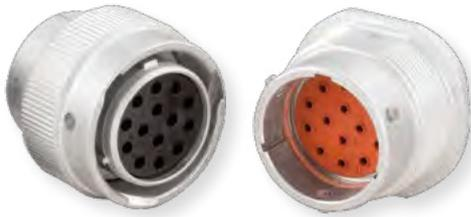
The DEUTSCH HD30 Series connectors are constructed from a metal shell developed to meet the needs of the heavy duty equipment and transportation industries. The HD30 features include quick connect-disconnect bayonet coupling, single hole bulkhead mounting, silicone seals, and a rear insertion/rear removal contact system.
