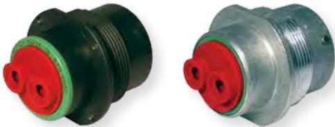
Originally designed for multiplexing and battery cable applications, the DEUTSCH C030 modification is an environmentally sealed, heavy duty two cavity connector that accepts size 4 solid contacts rated up to 100 amps for each cavity.
