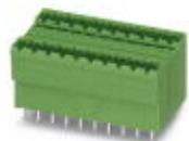
Header, Nominal current: 10 A, Rated voltage (III/2): 320 V, Number of positions: 3, Pitch: 5.08 mm, Color: green, Contact surface: Tin, Mounting: Wave soldering, In combination with MVSTB or FKCV plug components, both an MVSTBW (or FKCVW) and an MVSTBR plug (or FKCVR) must be used. Combination with TMSTBP plug components is not possible!
