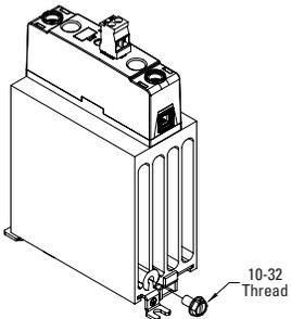
Protective earth (PE) screw type recommended is 10-32 UNC standard not provided with SSR. Through the use of a DIN rail ground (protective conductor) terminal block, the DIN rail itself can be used as the grounding bus bar. In this case, the zinc plated steel material used for the DIN rail clip of DR45 models, permits a secure path to ground and avoid the need of a further PE connection.
